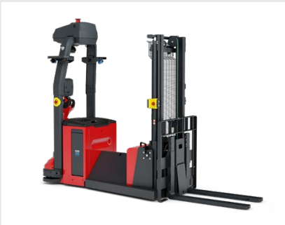
Flexible handling thanks to cantilever fork arms
